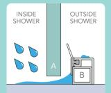
A - Sliding Door Glass B - Minimal Barrier Bar I - Threshold Seal
