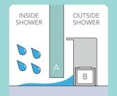
A - Sliding Door Glass B - Minimal Barrier Bar 2 - Threshold Bar
